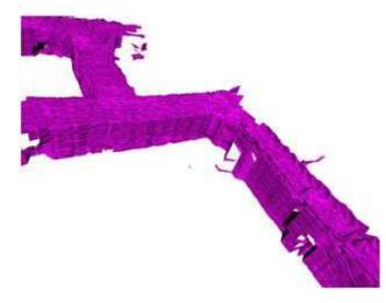
Figure 22.17: 3D indoor map from a swept vertical plane LADAR. Registration is from a horizontal LADAR using SLAM algorithms.
