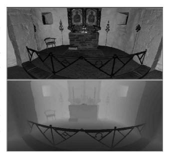
Figure 22.1: Above: Registered infrared reflectance image. Below: Range image where closer is darker.
