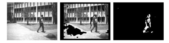
Figure 22.19: Independent motion detection from a moving platform. Reference image on left is forward-projected using the motion homography to the center image; right image is difference with actual image.
