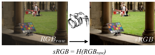
Figure 2: Color correction (mapping raw to display sRGB) is an homography problem. This figure is also a color chart example which was used for our color correction evaluation.
