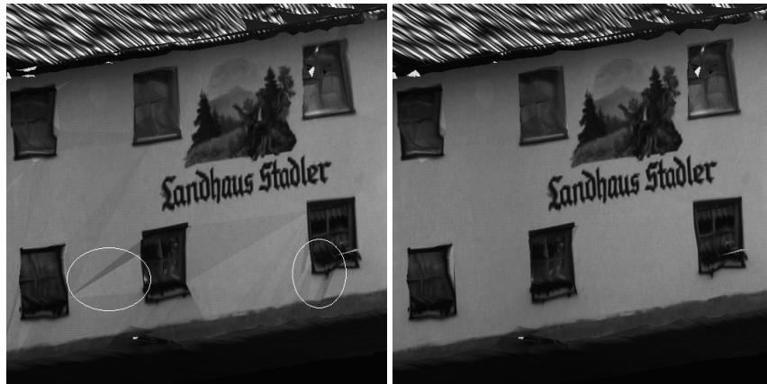
Fig. 3. A close view of a wall of the farmhouse. On the left is the unconstrained model. Surface ripples are most easily seen in the circled areas. On the right is the optimised model.
