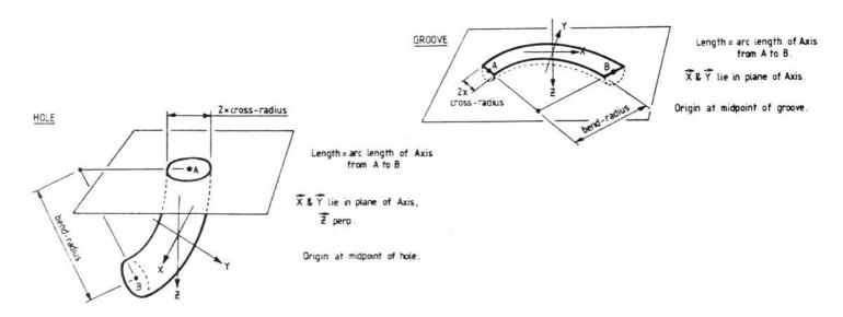
Figure 5: Definition of HOLE Feature
