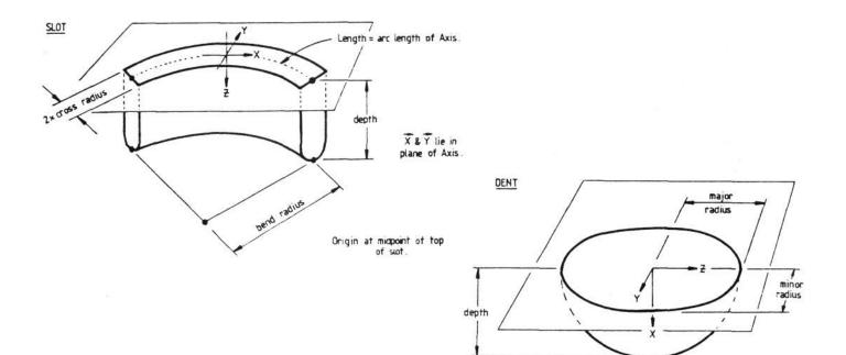
Figure 7: Definition of SLOT Feature
