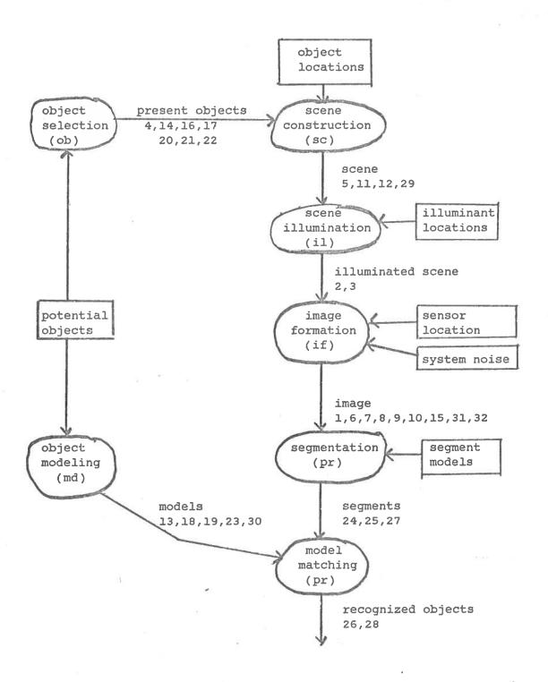
Figure 1 - image processing schema and anomaly appearance (numbers beside arcs refer to anomalies - see section 3)
