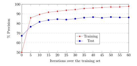
Figure 5: Training and test precision achieved by Nurbsnet after 60 training iterations using the ModelNet10 dataset with 2 internal Nurbs
