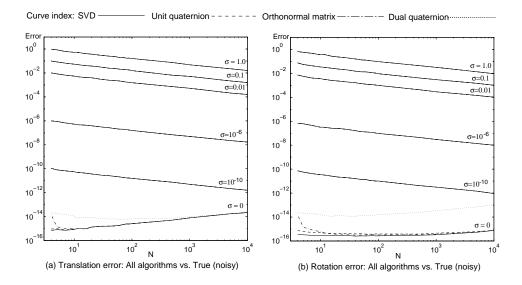
Figure 1: Errors between computed translation and rotation from algorithms and known transformation. Graphs (log-log scale) are translation error,  $\|\hat{T}_{alg} - \hat{T}_{true}\|$ , and rotation error,  $\|\hat{q}_{alg} - \hat{q}_{true}\|$ , vs. data set size, N.
