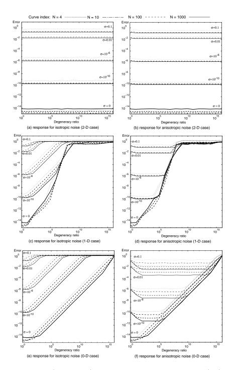
Figure 2: Graphs (log-log scale) of RMS errors of SVD algorithm for (a-b) 2-D, (c-d) 1-D, and (e-f) 0-D degenerate data sets of changing size under isotropic and anisotropic noise of varying levels.
