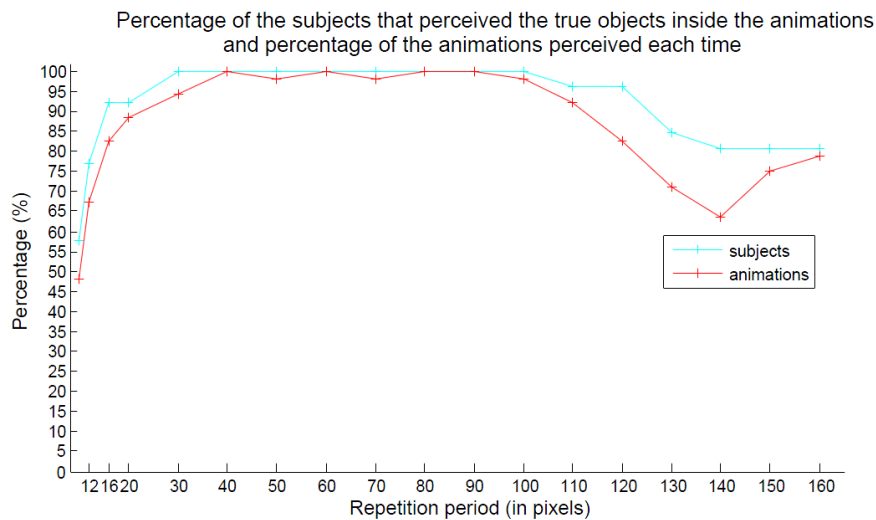
Figure 5.24: Percentages of the subjects that perceived the true objects inside the videos and percentages of the videos perceived correctly (true object) under different repetition period settings.
