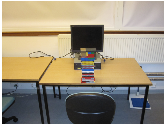
Figure 4.2: Front view of the experimental setting. The Lego chin support object with soft surface on top can be seen in front of the projection screen.
