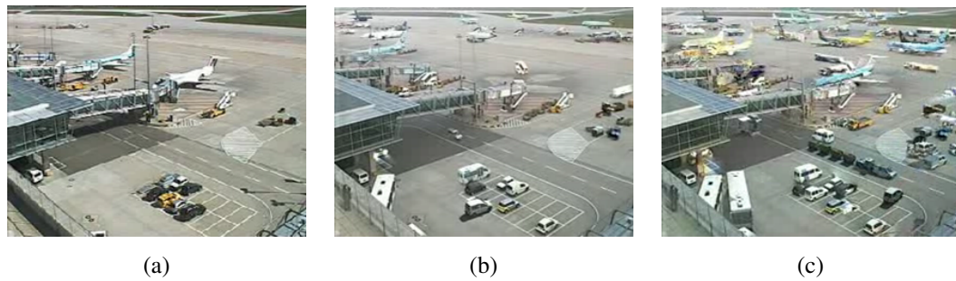
Figure 2.2: Video synopsis and indexing. Airport surveillance video. (Taken from [Yael Pritch and Peleg, 2008]) (a) Typical image. (b) Image from Synopsis video. (c) Video Synopsis at a smaller duration (more collisions between elements).
