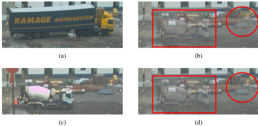
Figure 4.5: Ghosting. (a) and (c) are image segments with vehicles that cause the ghosting. (b) Independent color channel median. (d) Multivariate Median. Bounded regions show the defects. They are less evident in when MVM is used
