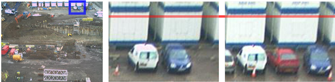
Figure 3.2: Jitter example between consecutive day images from Corinthian camera images. Red line shows the vertical movement of the camera.
