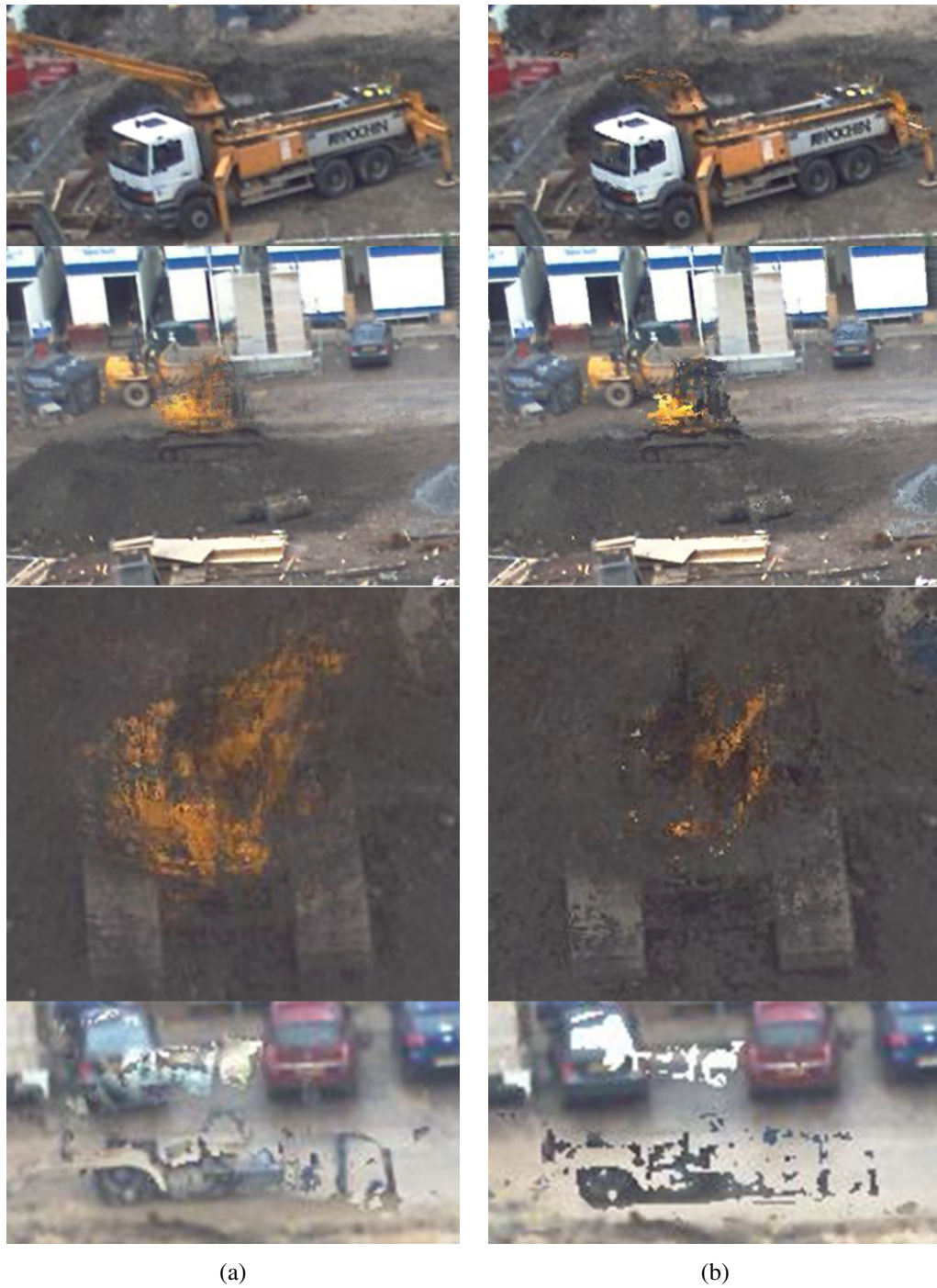
Figure 4.22: Enlarged day image segments for comparing processing methods. (a) Multivariate median filter. (b) Non-parametric Kernel density estimation filter.
