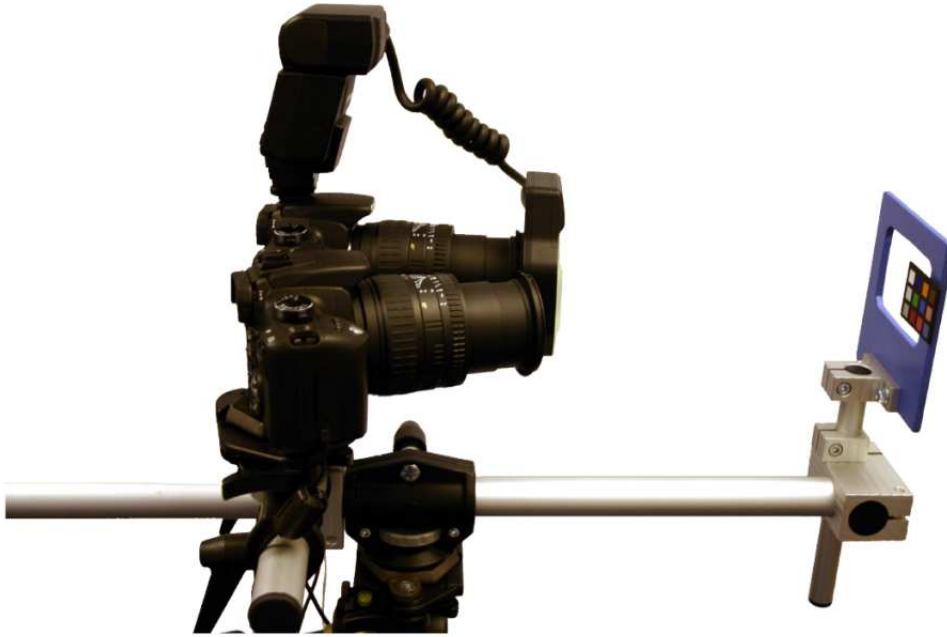
Figure 3.1: Stereo camera rig. Original image due to [37]
